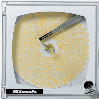
Ill.: Disc-type pen-recording thermometer for installation in refrigerators and freezers.
